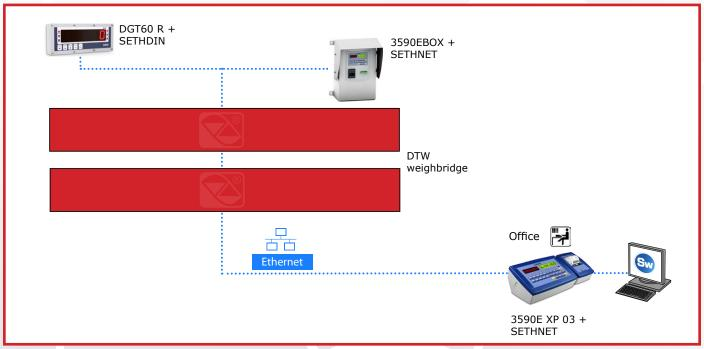
With this configuration, the weighbridge can be used from the office and in self-service mode when the office is closed.
