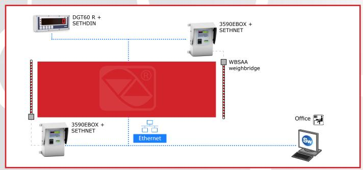
Thanks to the 3590EBOX, it is possible to run the weigh using the automatic identification number, the plate, or through RFID or BADGE.
